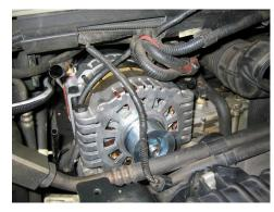
**10.** Rotate pulley by hand to verify that rotor spins freely. Install belt
