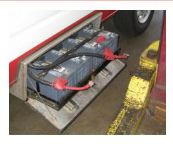
**1.** Disconnect batteries and remove existing alternator
