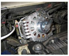
**8.** Install using the (3) spacer and bolts provided
