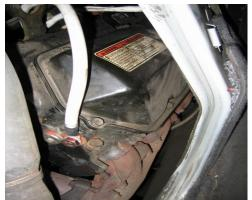
**14.** Connect negative cable to threaded boss on block
