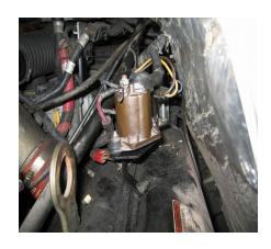
**5.** Install bracket provided in kit onto stud previous supporting air chamber box
