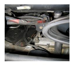
**4.** Remove glow plug relays and bracket
