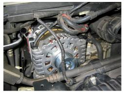
**9.** Tighten bolts to 25 ft.lbs. max. Apply thread-lock
