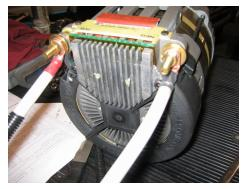
7. Attach cables and pulley prior to installing in vehicle
