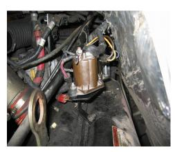
**13.** Route negative cable towards cab alongside solenoid and bracket
