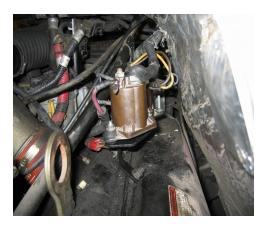
**6.** Install both solenoids on the new bracket
