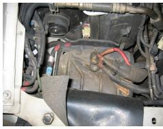
**11.** Locate battery junction block in left front of vehicle
