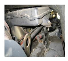
**3.** Remove air chamber box and support brace
