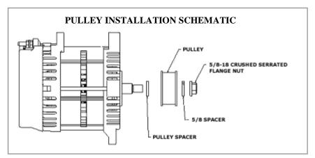
alternator pulley to the overall clearance length to determine available length for the Eco-Tech Alternator. The fit length required for Eco-Tech Alternator is 9". The existing alternator pulley will interchange and Alternator belts will align properly.
