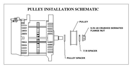
overall clearance length available to determine space for the Alternator. The new alternator pulley that comes with the kit will mount, so that the Alternator belt can be reused and will align properly.
